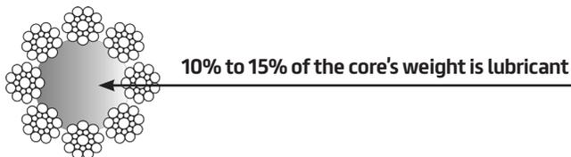
During manufacturing, a low-viscosity lubricant is applied to the sisal and strands of the ropes. The main purpose of the lubrication is to give 'life' to the rope's working parts and allow traction to take place. This lubricant also reduces metal-to-metal friction when the rope is operating and helps inhibit rust formation. It typically accounts for 10% to 15% of a sisal core's weight.
