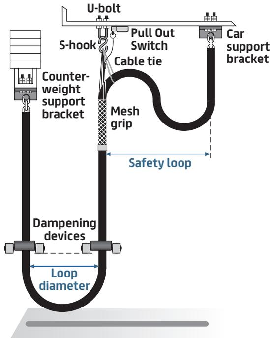
One connection location is the car support bracket used to terminate the cable to the car and the other is for locating an S-hook that provides a "mechanical fuse" for the cable.
